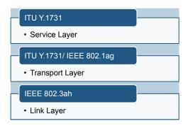
The TX130M+ offers a complete tool set for Link Level (IEEE 802.3ah) and Service Level (IEEE 802.1ag/ ITU- Y.1731) OAM for monitoring and maintaining carrier grade Ethernet services.
