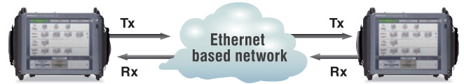
Running Service Activation Test in local – remote configuration using two MT1100A testers
