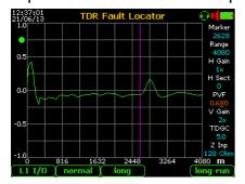
location of possible faults or anomalies as: interruptions, short circuits, low insulation, bridge-taps, split-pairs, and also the possible micro-interruptions thanks to the "Sample & Hold" test modality.
