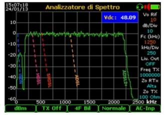
The ACT6000's **Spectrum Analyzer** can operate on various frequency bands, readout mode and also with special Front/End configuration as the High Impedance.
