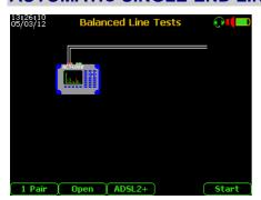
Adopting the optional ASW-1 software, after the quick cable selection among the many types included on the data base, it is possible to start an Automatic Sequence to perform a complete set of electrics and transmissive tests to qualify the line for a specific service.
