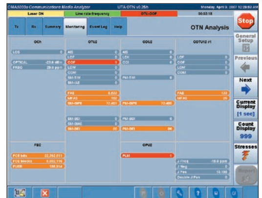
OTN Error and Alarm Display Showing Each Network Layer
