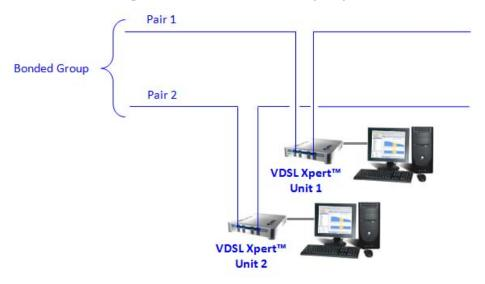
Start the capture with the first VDSL Xpert unit, and then start the capture on the second VDSL Xpert unit before the first modem reaches Showtime.
