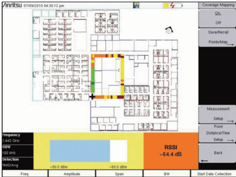
Figure 24. Plotting signal strength to find an interference source.
