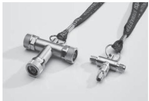
Figure 3-11. Convenient calibration components for the VNA provide the Open, Short and Load standards for the SOLT calibration procedure.
