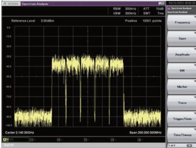
Figure 27 : Spectrum analyzer MS269xA/MS2830A - Example of Spectrum of LTE-Advanced signal (Component Carrier: Bandwidth 20 MHz, 5CC)
