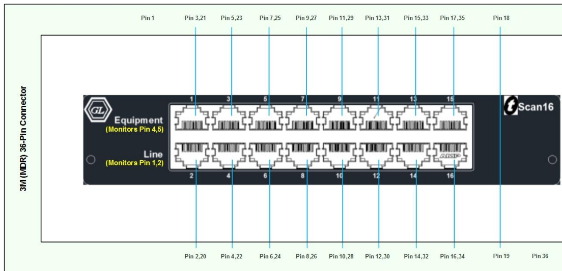
Figure 2: MDR 36-pin Connector to tScan16™ Breakout Box- Pinout
