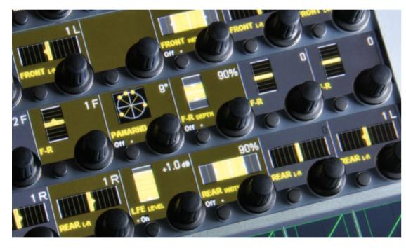
Key parameters can be adjusted directly via touch on the Vistonics screen without the need to spill single mono or stereo channels to additional faders.
