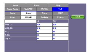
VoIP Call Expert – Emulates an IP phone to place and receive calls using SIP or H.323 protocols. Real-time evaluation of voice quality with a complete set of measurements is available at the end of the call, including packet statistics, jitter statistics, and MOS and R-factor call quality scores. Support VoIP trunk test with bulk call generation of up to 24 simultaneous calls.
